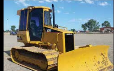
CAT D5G LGP DOZER C/A W/ 6 WAY BLADE
