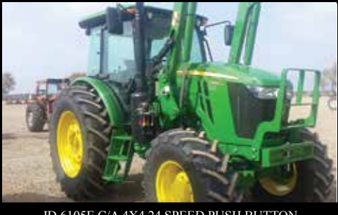
JD 6105E C/A 4X4 24 SPEED PUSH BUTTON W/REVERSER W/H310 LDR- NEW TRACTOR
